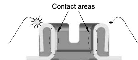
Contact areas are not exposed to the outside penetration of the flux or other physical particles.
