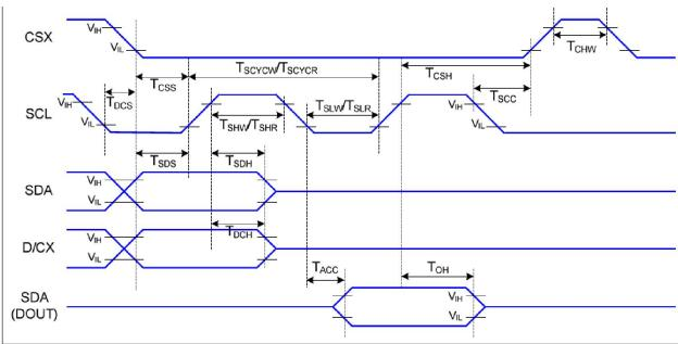
Figure 8.4.1 4-line serial interface timing
