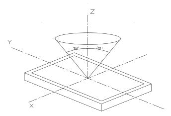
Inspection should be performed within angle  $\phi$  ( $\phi$  is usually 30°) from Z axis to each X and Y. Inspection distance in any direction within  $\phi$  must be kept 30±5cm from the display surface.
